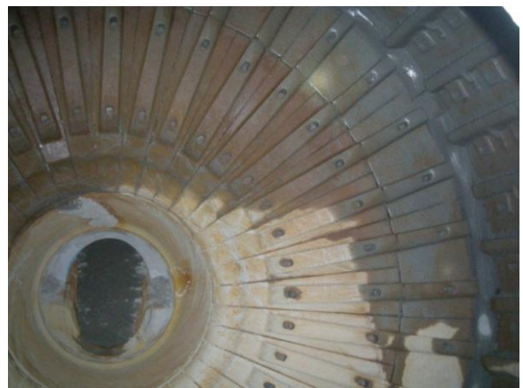
图四 端衬板磨损位置 Fig.4 Abrasion Conditions of End
