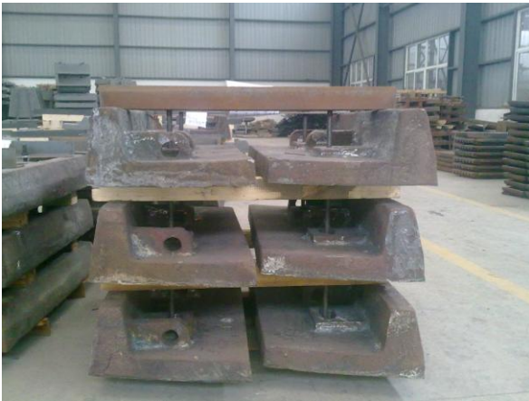
图三 矩形设计的半自磨机筒体衬板 Fig.3 Cylinder Liners with Rectangular
